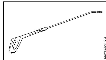
Use the long, angled spray lance only directly on the spray gun. Do not install a spray lance extension.
