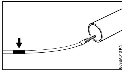
There is a mark on the cleaning hose underneath the nozzle (see arrow).
